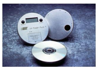
radiometer, the operator can immediately quantify the process. After product is cured satisfactorily, the operator exposes the radiometer to the same UV process. The UV level readings are displayed on the radiometer.
