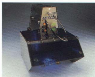
SS5109 UV Safe Enclosure with safety interlock prevents shutter operation when enclosure is open. The fixture holds the light wand for hands free operation.
